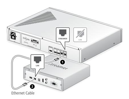
The Streamer Port provides a wired network connection for streamers, wireless speakers and other network audio products.
