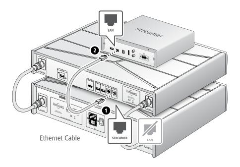
The Streamer Port provides a wired network connection for streamers, wireless speakers and other network audio products.
